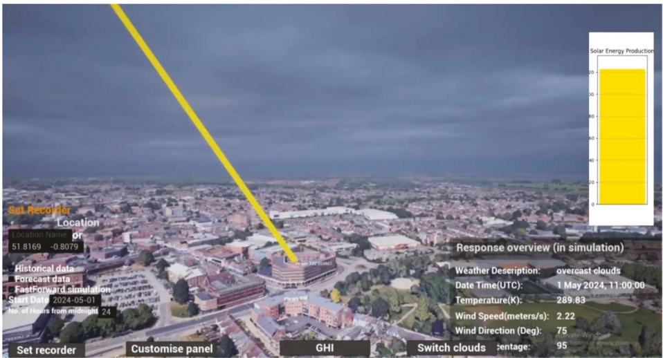
Figure 2. A snapshot of the Photovoltaic Digital Twin simulation.
