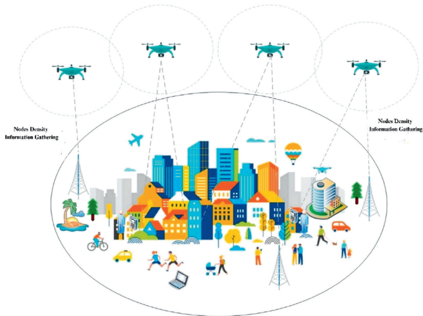
Figure 2. Estimating the density of IoT Network Nodes using Unmanned Aerial Vehicles (UAVs)
