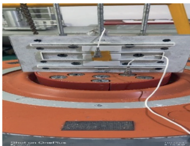
Figure 12. Position of Y-axis vibration on the shaker
