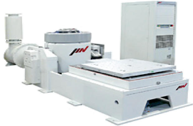
Figure 10. Vibration shaker model :i220 samsact testing services
