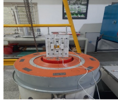
Figure 13. Position of Z-axis vibration on the shaker
